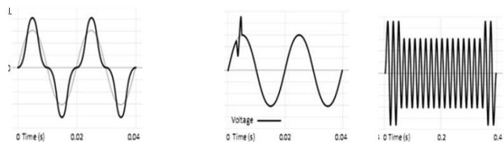
Figure 1. Possible disturbances due to (a). Fluorescent light load (b). Capacitive load (c). Overload (Industry Guide)
