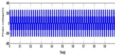
Figure 3a. Stator voltage – DPWM scheme
