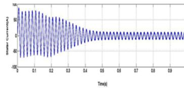
Figure 3b. Stator current – DPWM scheme
