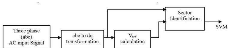
Figure 12. Block diagram – SVPWM pulse generation
