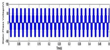
Figure 7a. Stator voltage – SPWM scheme
