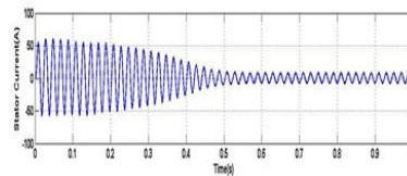
Figure 13b. Stator current – SVPWM scheme
