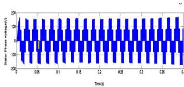
Figure 13a. Stator voltage – SVPWM scheme
