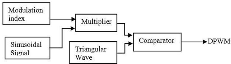
Figure 2. Block diagram – DPWM pulse generation
