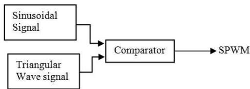
Figure 6. Block diagram – SPWM pulse generation
